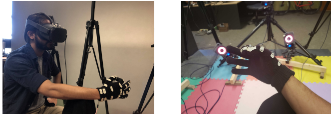
Fig. 2: The tracking setup consisting of 13 Vicon cameras and a felt glove with IR tracking markers attached.
